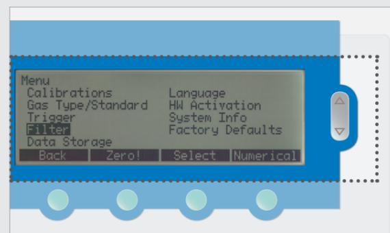
The display light contrast can be adjusted to your preference and viewing angle by pressing and holding the first button from the left then use the arrow key to select the desired contrast level.
