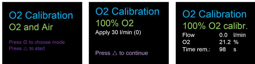
Figure 26: Screen displays "Calibration Oxygen and Air"
