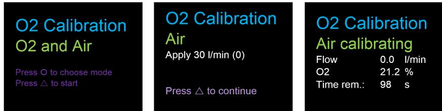
Figure 25: Screen displays "Calibration Air"
