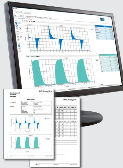
View your flow, pressure and volume measurements comfortably on your computer monitor, while simultaneously saving respiratory parameters.
