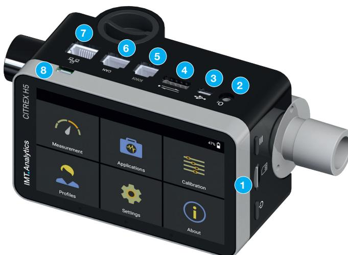
Figure 9: Electrical interfaces
